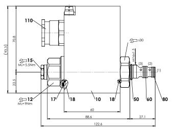
Dimensions of the solenoid coil see data sheet 1.1-183
