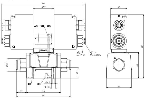
Dimensions of the solenoid coil, refer to data sheet 1.1-183 and 1.1-184
