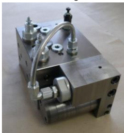
Hydraulic Block with an intensifier integrated
