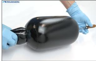
Use the threaded rod to guide the gas valve stem through the gas-side bore. Pass the nameplate and then the retaining nut over the threaded rod to the vessels face end. Loosely screw the retaining nut onto the gas valve stem and do not tighten it yet. Remove the threaded rod.
