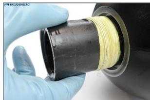
Fill the bladder slowly with nitrogen using the testing and filling device so that the bladder can gradually unfold during expansion and mold smoothly against the inner vessel surface. The gas filling pressure should not exceed 1 bar and the bladder should just touch the poppet valve of the fluid housing assembly.
