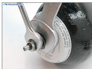
At the oil end, center the fluid port and its anti-extrusion ring again, creating an even contact with the vessel seat and a constant circumferential gap height between the fluid housing shell and the vessels locating bore. Hold the housing in position. Continue to fill the bladder until it exerts sufficient pressure on the poppet valve to prevent the fluid port housing assembly from shifting during the subsequent assembly steps. The filling pressure should not exceed 3 bar.
