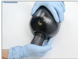
Remove the sealing, support and back up ring from the fluid port housing and take them out of the vessel.
