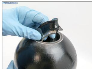
Remove the fluid port housing through the vessel opening .
