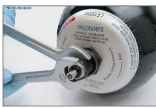
Insert and guide the fluid port housing assembly through the oil-side vessel bore with the collar oriented towards the gas end and place it inside the vessel. If applicable, disassemble the side drain plug first.
