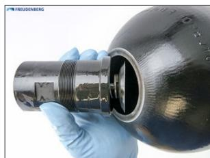
Pull the bladder out of the accumulator. Surface damage during extraction must be prevented in case of reuse of the bladder.
