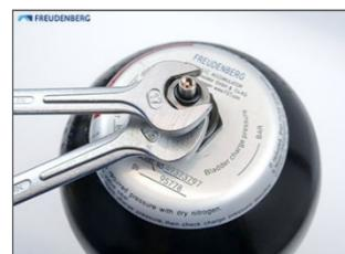
Unscrew and remove the retainer nut with countered gas valve stem.
