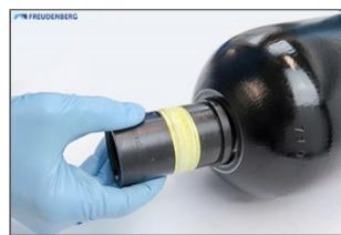
Re-lube the oil-side locating bore. Fold the anti-extrusion ring slightly and insert it through its locating bore into the interior of the vessel as carefully as possible.
