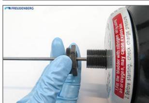
Screw in the gas valve body with its pre-assembled valve core and sealings. Tighten the valve body to  $14^{+2}$  Nm while locking the gas valve stem with a wrench.
