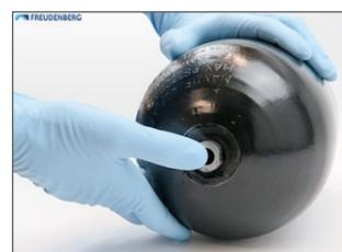
Carefully push the free gas valve stem inside the vessel until the bladder detaches from the bottom of the vessel.
