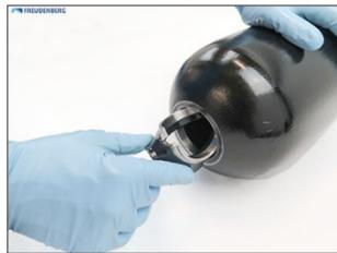
Put the anti-extrusion ring inside the vessel onto the fluid port housing with its contact surface aligned with the collar of the housing.
