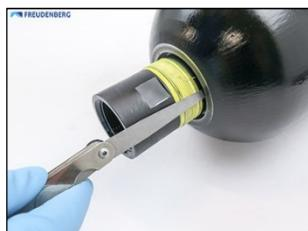
Carefully guide the chamber ring (only for accumulators from 10L), then the O-ring and finally the support ring over the threaded end of the fluid port housing using an O-ring lifter (or a similar tool) and mount it in the gap between the vessel and housing shell surface. Shift the rings axially up to the anti-extrusion ring without twisting or crushing the O-ring.
