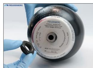
Remove the name plate and keep it in a safe place.
