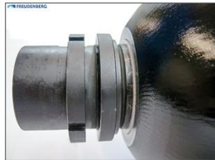
Screw the groove nut onto the thread of the fluid port housing and screw it hand-tight with the spacer ring. Then tighten the groove nut with countered fluid port housing using a hook torque wrench and apply the recommended torque according to the drawing or specification Cf. 4.1.
