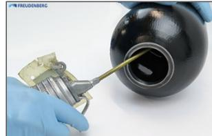
Slightly squeeze the bladder at its head end, insert it through the opening on the fluid side and push it step by step inside the vessel. Make sure that the bladder does not twist or bend.
