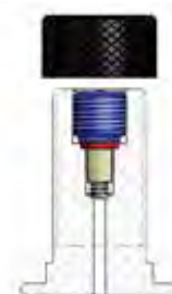
Model of valve stem integrated 5/8" 18 UNF (D)
