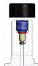
Model of valve stem integrated 5/8" 18 UNF (D)
